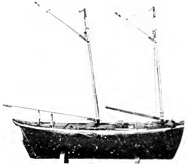
SMALL CHEBACCO BOAT, 1790–95, a type much used in the Massachusetts inshore fisheries from 1785 to 1815. This old and somewhat crude rigged model (USNM 39198), of indeterminate scale, shows the basic features of a small boat of the type. ( Smithsonian photo 44697-c. )
